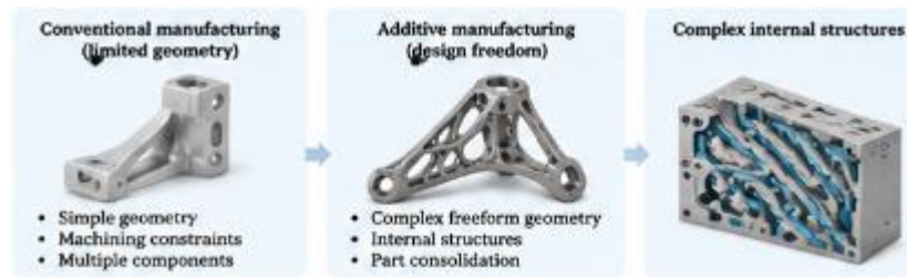
Figure 3. Topology optimization-based design workflow for additive manufacturing
