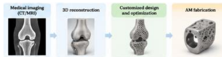
Figure 5. Workflow of patient-specific biomedical design enabled by additive manufacturing
