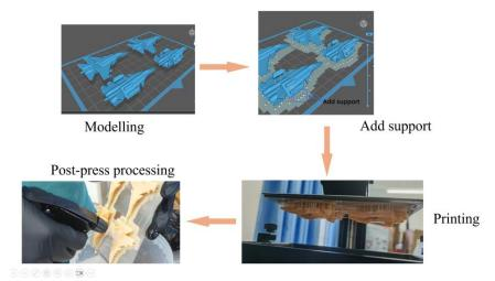
Figure. 12. 3D Printing Flowchart
