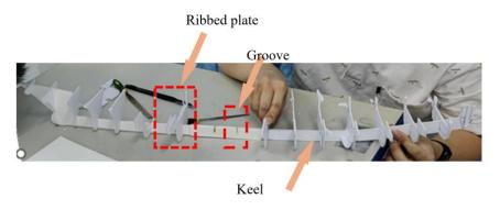
Figure. 9. Hull frame.
