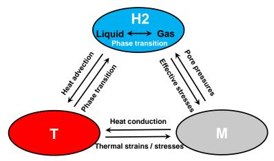
Figure. 1. THM coupled processes of unsaturated soils.
