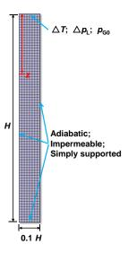
Figure. 2. Mesh division and boundary conditions of the verification model
