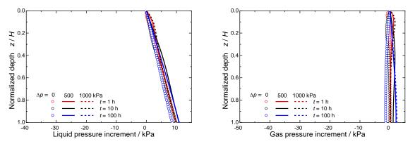
**Figure. 8. Comparison among different initial pore pressure:** (a) liquid pressure increment; (b) gas pressure increment.
