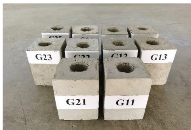
Figure. 2 Rock mass reinforced by cement slurry after drilling
